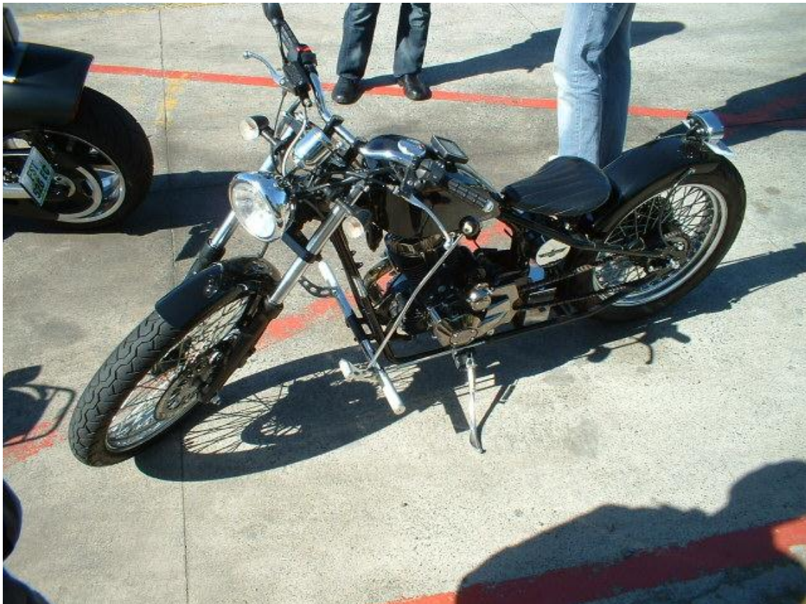
Another unusual unit was this chopper, also a 250cc capacity, solid frame with a gear lever attached to the foot support.
